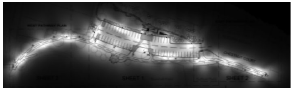
Illumination pattern of the new solar powered walkway lights along the Playstead.
