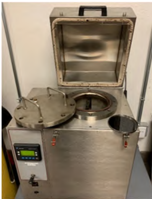
Fig. 8. Pressure aging vessel (PAV).
