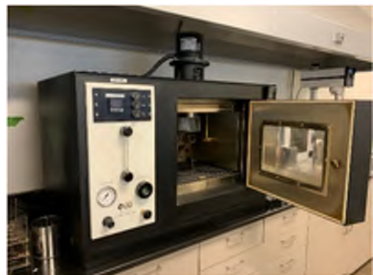
Fig. 7. Thin film oven aging.
