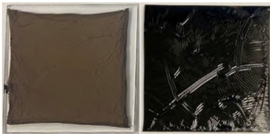
Fig. 2. Pictures of asphalt binder (AB1) after 2.5 \times 10^3 J_{340 \text{ nm}} of simulated sunlight exposure in the water-submerged (left) and open atmosphere configurations (right).
